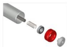
RODILLO UNIVERSAL HEXAGONAL RETRACTIL VISTA EXPLOSIONADA
